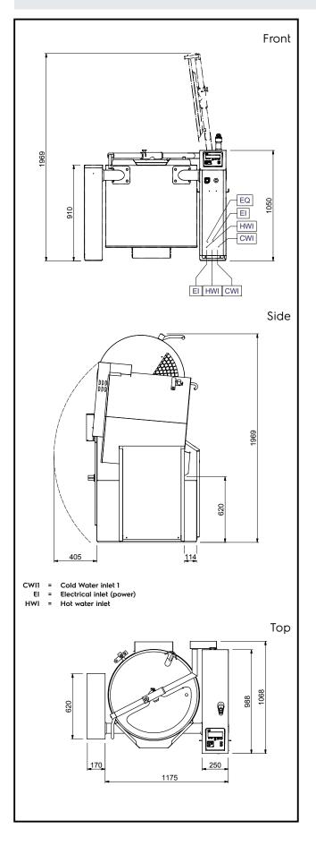
High Productivity Cooking Smart Electric Boiling Pan 2001t, 600mm tilting height
